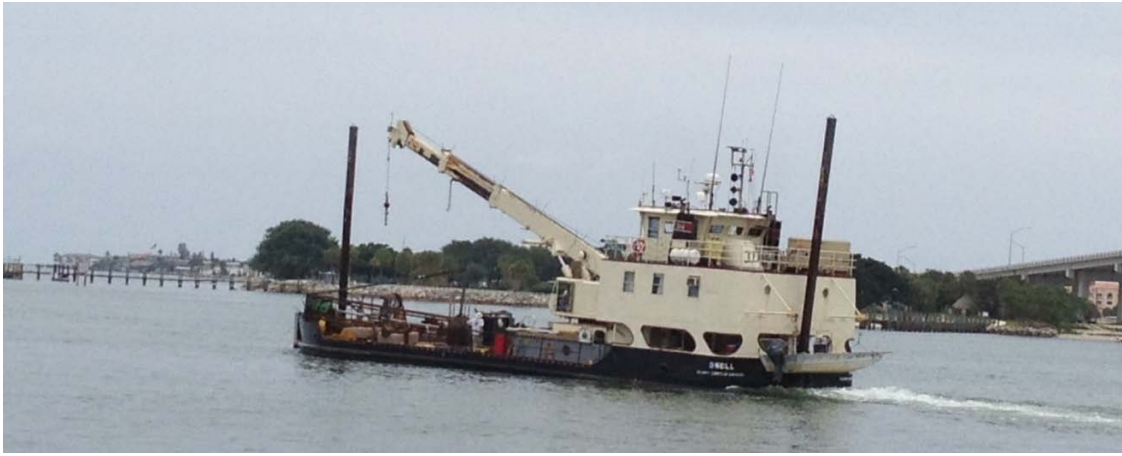
Above: USACE Wilmington District's D/B Vessel "SNELL" is a 104'x 32' vessel drawing 6' of water, equipped with a 35 ton crane capable of multiple functions from drilling to dredging and dock/snag removal.
