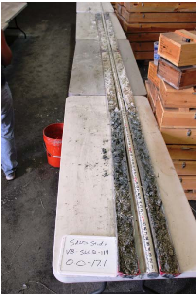
Below Left and Right: Core showing penetration through rock; 12.5 feet of moderately hard limestone was recovered. The material was moderately weathered, clayey and broken by drill action.
