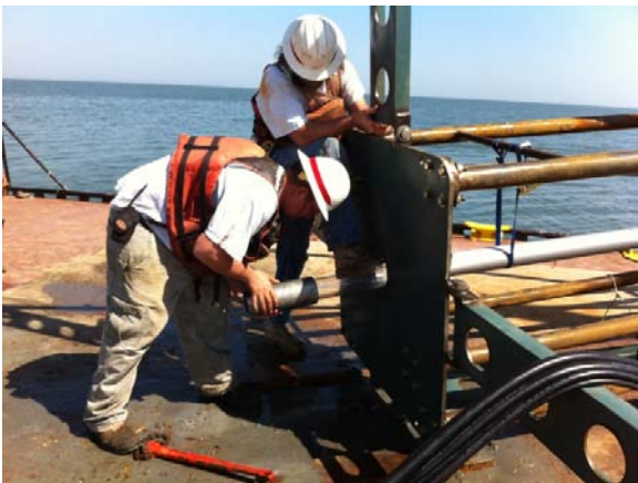
Above Left: The nose cone treads onto the vibracore liner preventing material from entering the annulus between the liner and pipe.
