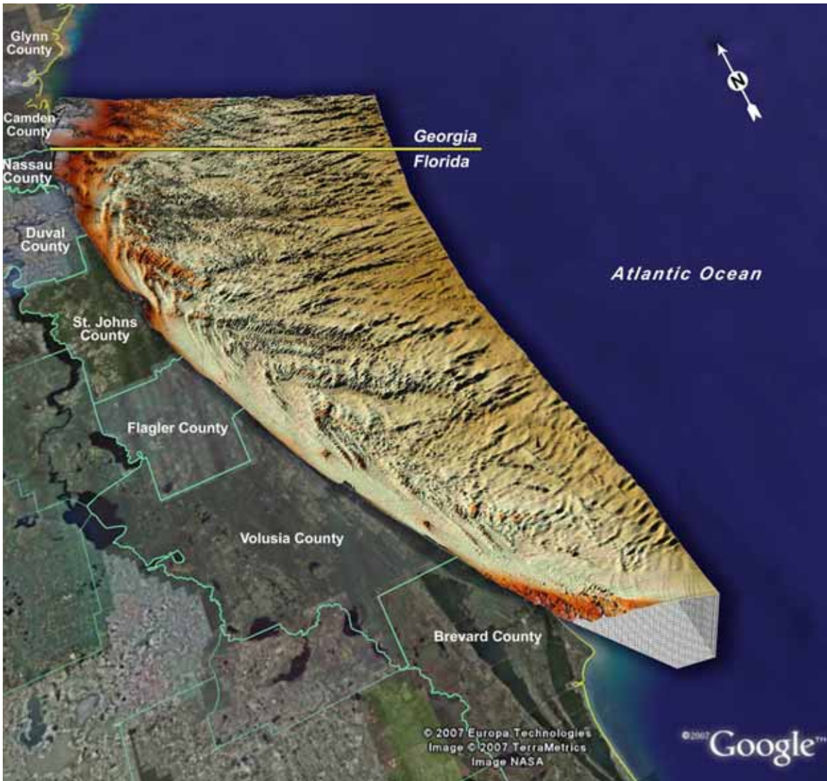
Figure 3-3. Composite diagram (not to scale) showing the study-area terrain model in relation to cadastral boundaries superimposed on satellite imagery. Near- and offshore sand ridges, bars, banks, shoals, and sand waves are clearly evident in the color-ramped bathymetry. Cape Canaveral is the large salient feature in Brevard County.
