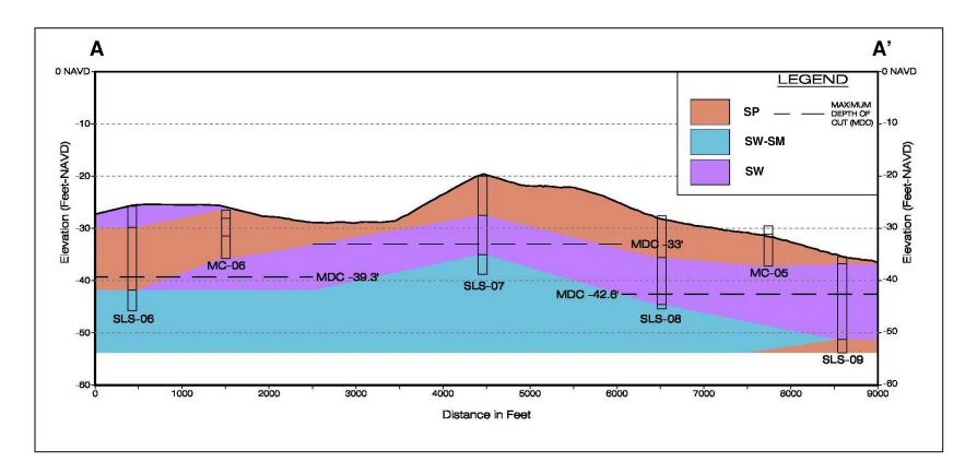
Figure 5.7: St. Lucie Shoal: Area A – Interpreted Fence Diagram
