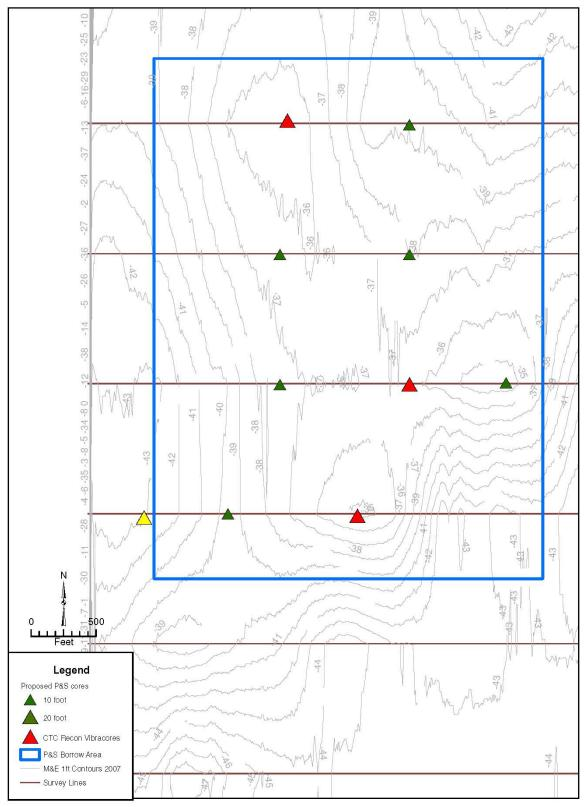
Figure 6.5: Proposed Plans and Specs Vibracoring Plan: Area D
