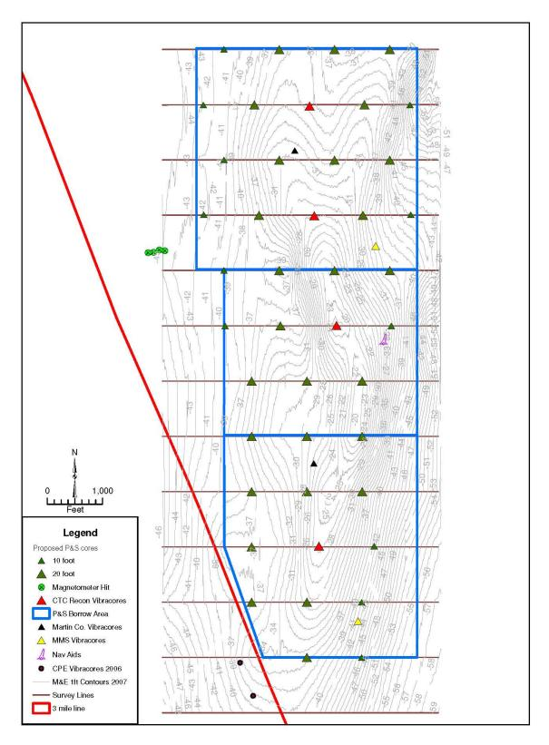
Figure 6.2: Proposed Plans and Specs Vibracoring Plan: Area A
