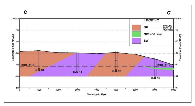
Figure 5.10: St. Lucie Shoal: Area C – Interpreted Fence Diagram
