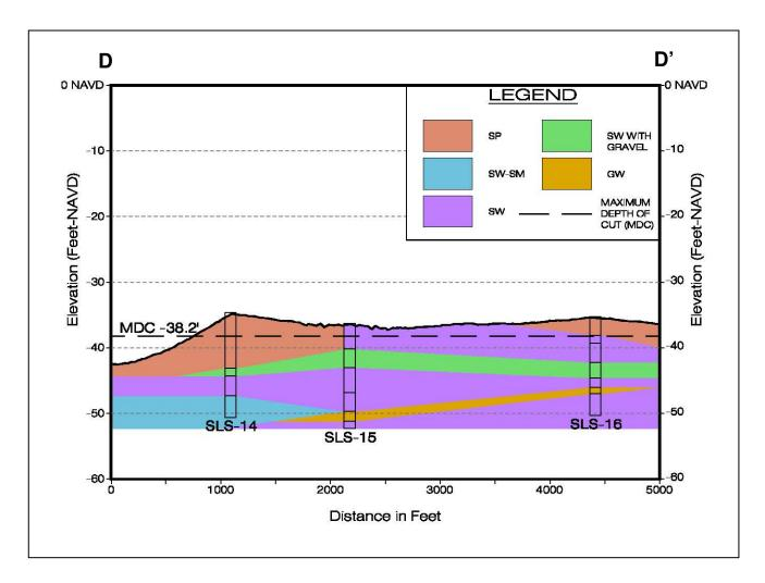
Figure 5.13: St. Lucie Shoal: Area D – Interpreted Fence Diagram
